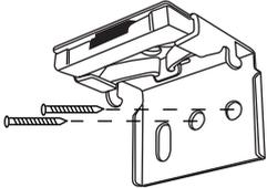
1. Position the end brackets for fixing (either face or top) ensuring that the brackets are fixed approximately 50mm from the end of the blind. The centre bracket (required for blinds exceeding 1200mm width) may be positioned as required.
