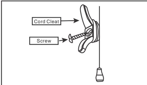
Cord cleats must be installed to comply with Regulations.
